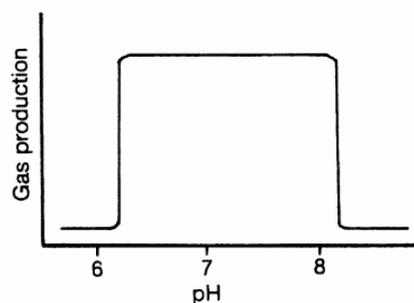
The effect of pH on biogas production.
