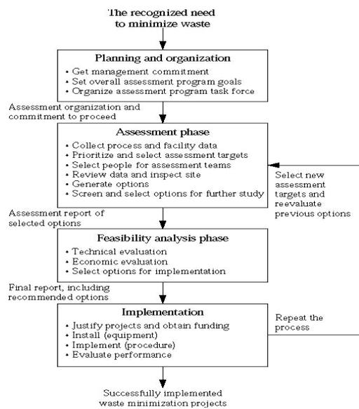
Figure 7.3 EPA's waste minimization assessment procedure (LaGrega *et al.*, 2001)
