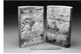
Cross-section of macroencapsulated heterogeneous debris in phosphate ceramics.
